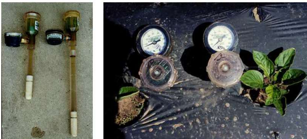
Figure 15: Tensiometers are often used to measure suction in unsaturated soils.
